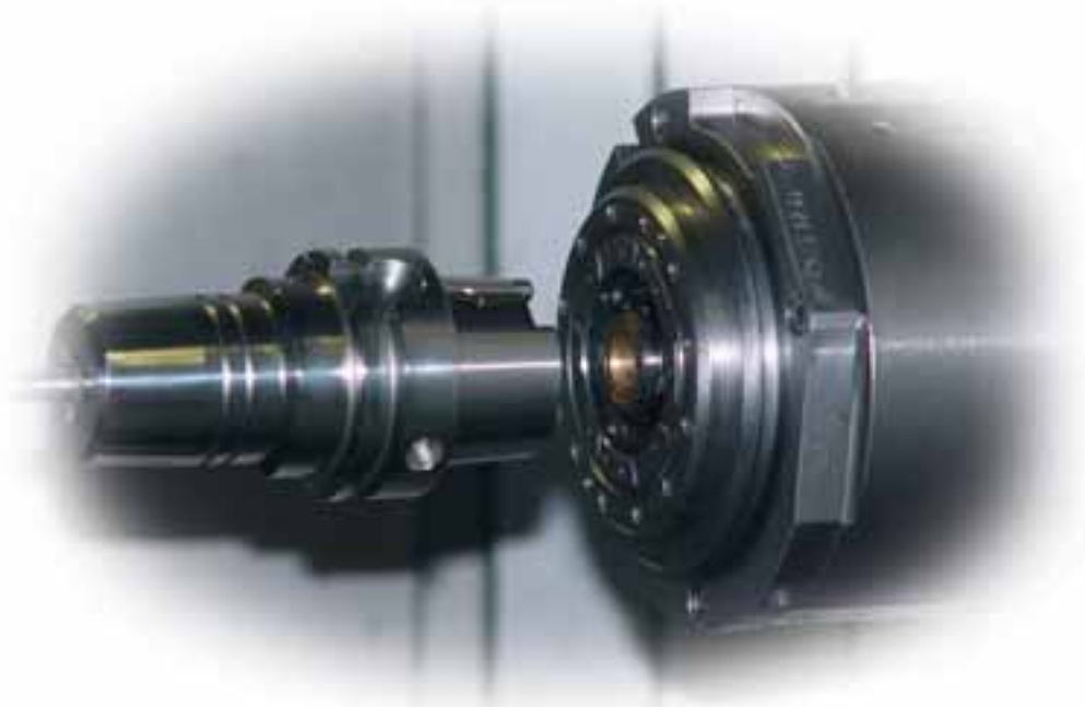
Fig. 1: HSK-A 63 interface, automatic tool change
