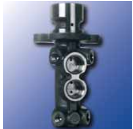
Safety component: Drilling and reaming of a master brake cylinder
